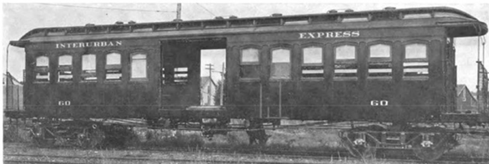
OLD MANHATTAN ELEVATED CAR REBUILT FOR EXPRESS AND FREIGHT SERVICE, WESTERN OHIO RAILWAY
